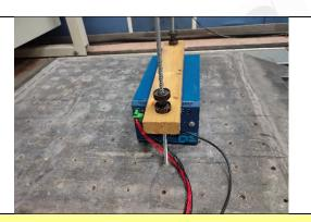
Mechanical Shock Test (±X axis)
