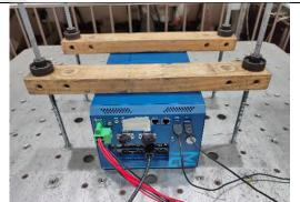
Vibration Test (Z axis)
