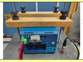
10. Mechanical Shock Test (±Z axis)
